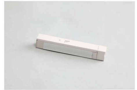
In-line touch dimmer Option 1: stepless dimming 5%-100% Short touch for on/off, long touch for dimming Option 2 3-step dimming 10%-50%-100% Short touch for different states off-10%-50%-100%-off . . ]Max. 72W/24V in a row]
